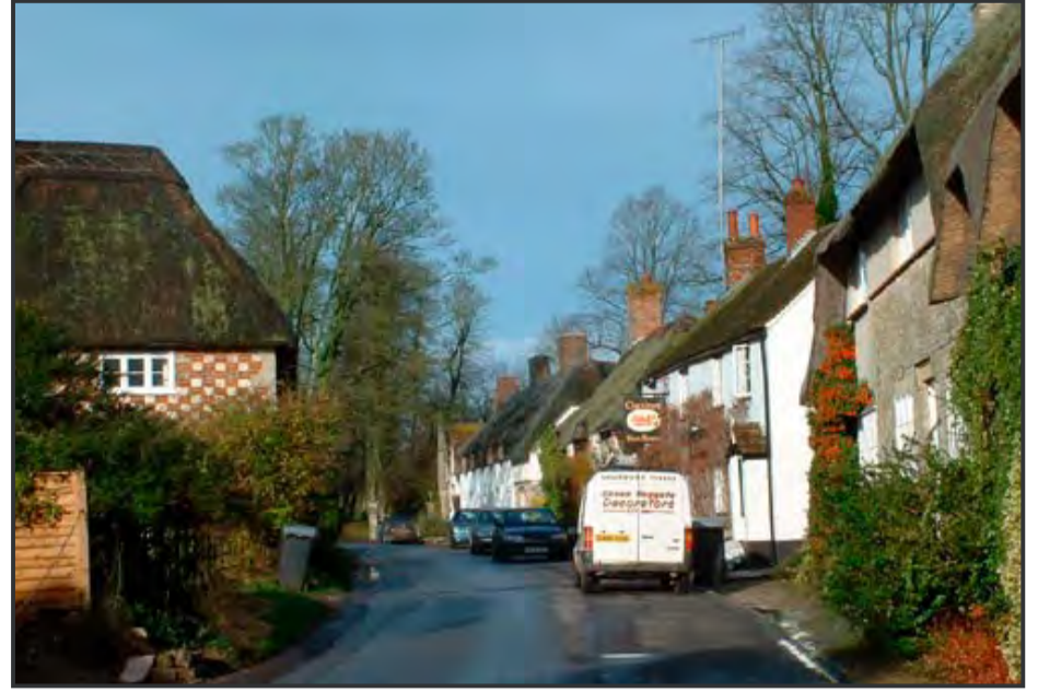
The shortage of building stone is reflected in 'chequerboard' patterns of stone knapped flint. Thatch is also common.
